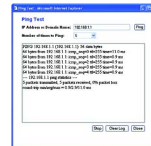
Figure 6-40 : Ping Test (Test Ping)
