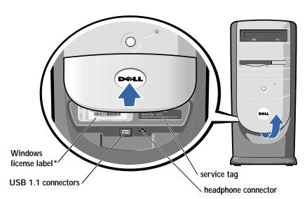
HINT: To prevent damage to your computer, the front door is designed to "break away" if it is lifted up too far. For instructions on how to reattach the door, see
