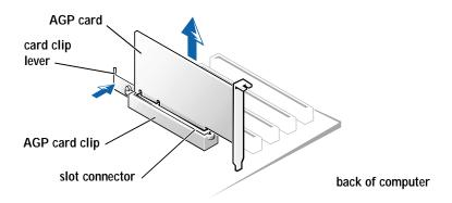
To replace the AGP card, gently press it down into the slot connector until it clicks into place. Press the card clip lever while inserting the card into the slot connector.
