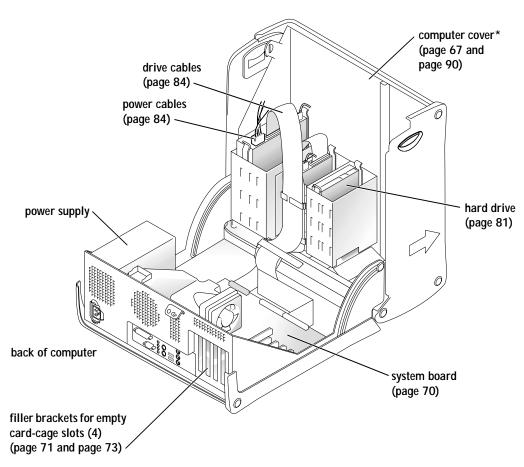
Depending on the types of drives installed in your computer, the cover may not open as widely as shown in the figure.
