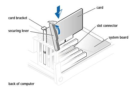
Ensure that the card is fully seated in the connector.
