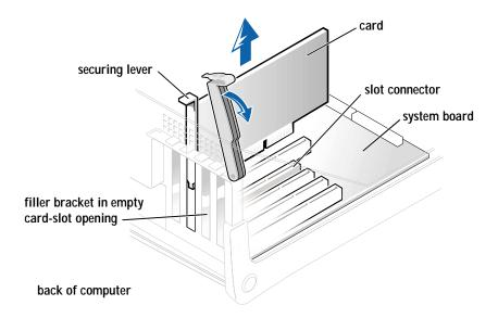
8 If you are not replacing the card, install a filler bracket in the empty card-slot opening.
