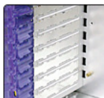
Screw-less PCI fingers, easy to install
