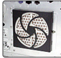
80mm cooling fan with air filter in front (intake)
