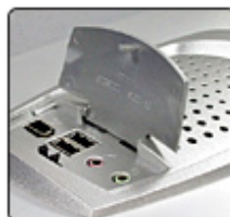
Dual USB2.0, IEEE1394 Firewire, audio & speaker ports
